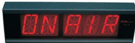
The new AAL-03 On Air Light features a 10 word user programmable memory. A word of up to 6 characters or sequences of words can be displayed in various states and speeds. Features: 10 word memory, 6 character LED display, Steady or flashing display, Adjustable flash speed and Adjustable word transition speed
